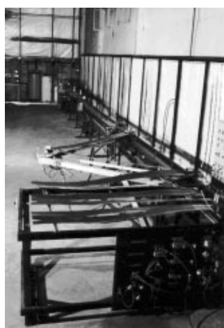
Sunstrip™ FAKIR Operation: uncoil, punch, inflate, and bend SS146/8 fin into serpentine absorbers
