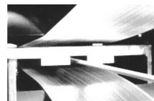
Brushed aluminum and copper before roll bonding process
