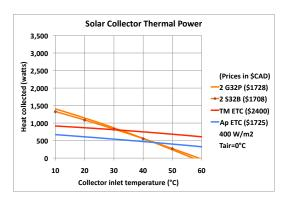
One graph is for solar radiation of  $800 \text{ W/m}^2$ , a sunny day, and  $20^{\circ}\text{C}$  air. The same information has been plotted also for poor solar conditions: solar radiation of  $400 \text{ W/m}^2$ , which is somewhat cloudy, and  $0^{\circ}\text{C}$ . The Thermo Dynamics G32P and S32B, outperform the AP-30 for
